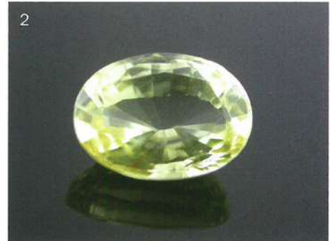
This synthetic sapphire of 2.14 ct contains fine milky zones resembling those common in sapphires of natural origin.
