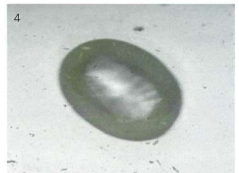
The synthetic sapphire shown in 2, which here shows transparency to SWUV radiation. Note the transparent centre and dark edges.
