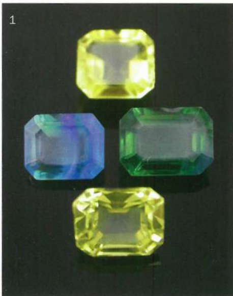
The four synthetic sapphires obtained for reference and the subject of this study. Note the sheen effect restricted to the table facets, a feature commonly displayed by natural sapphires. Also note the curved zones in the greenish-blue stone. Weights 2.10–3.41 ct.
