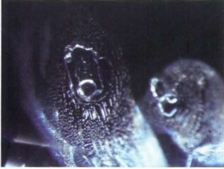
Melted crystals (evidence of high temperature heating) in a beryllium-diffused blue sapphire examined in GIA Laboratory, Bangkok. Photo K. Scarratt © GIA
