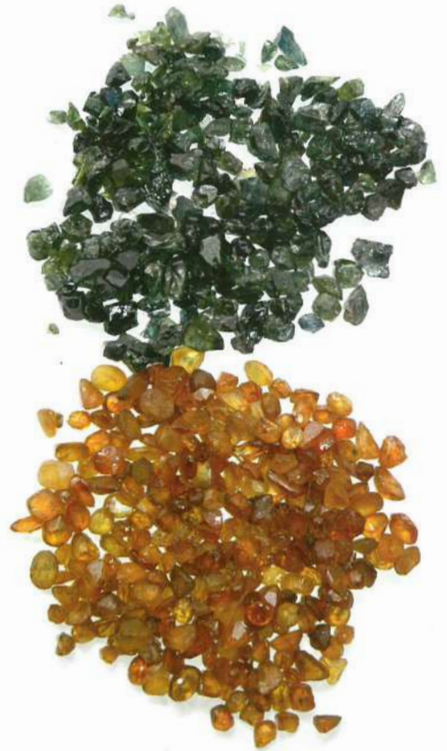
Green sapphires before and after beryllium treatment, clearly showing the dramatic change of colour.
