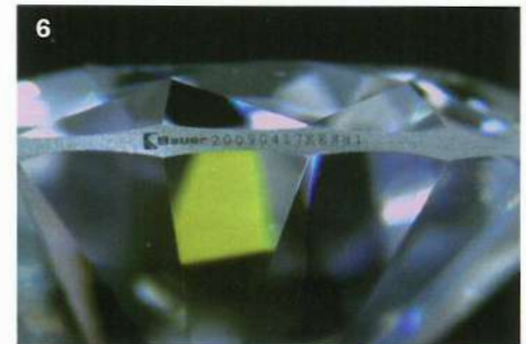
4: The laser in action (circled). 5: The laser inscription applied to the girdle. 6: The finished product.
