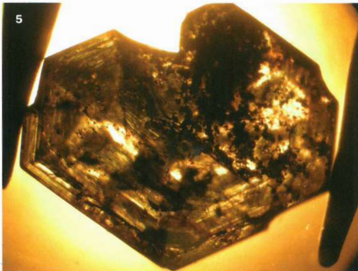
View parallel to one of the cubic three-fold axes of a demantoid crystal; growth zoning parallel to dodecahedral and trapezohedral faces. Immersion, magnified 25x.
