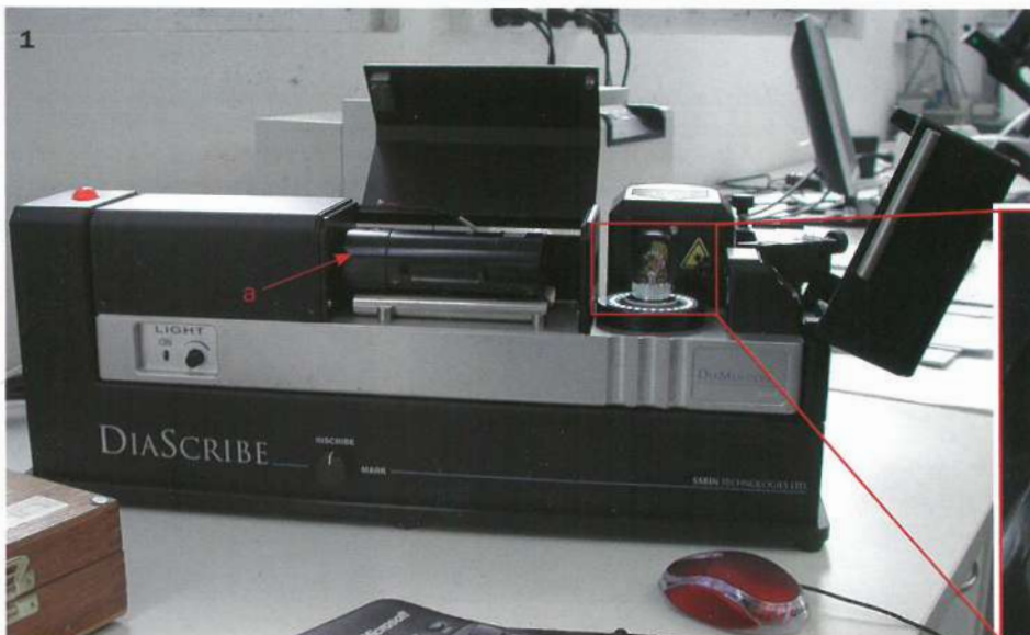
1: The Sarin Technologies DiaScribe. a. Interchangeable lenses b. Stage c. 70x viewer d. Laser.
