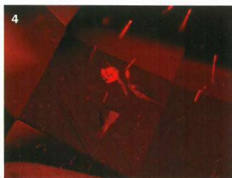
4 Six-sided metallic platinum flake and short hollow tubes have been found in one of the flux synthetic red spinels. © H.A. Hänni, SSEF 2008.
