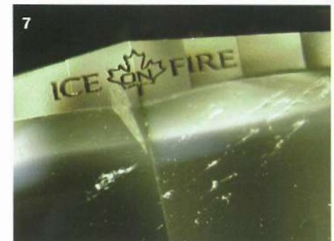
7: No damage was done to this diamond, despite the laser inscription being carried out on top of a surface-reaching feather.
