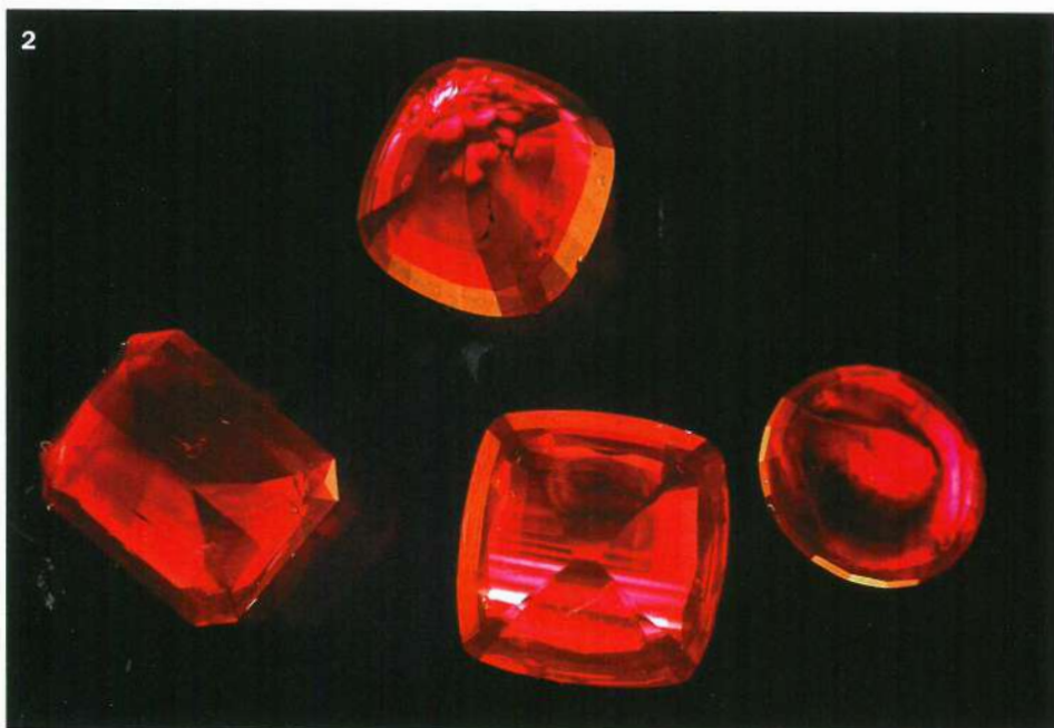
2 The flux synthetic spinels under the polariscope showing anomalous extinction, which may also be seen in natural spinels. © M.S. Krzemnicki, Swiss Gemmological Institute SSEF.
