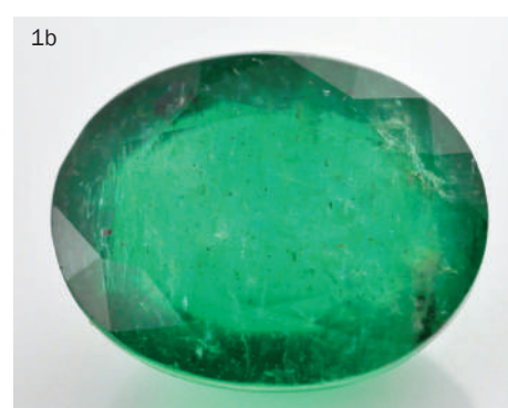
The two specimens identified as composites (1a weighing 2.64 ct and 1b 7.58 ct) consisting of light coloured beryl and deep green glass.
