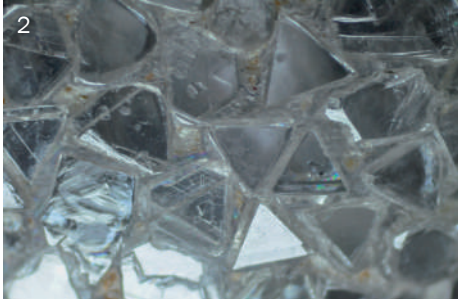
2: Individual diamond chips displaying a range of shapes with an adamantine lustre. Note the dull whitish matrix and yellowish to brownish substance. Magnified 45x.
