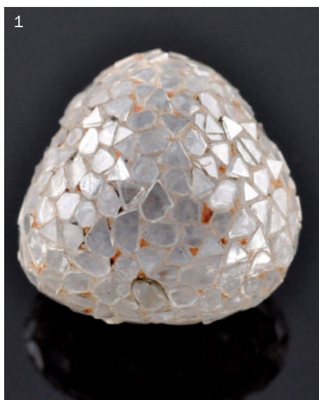
The 38.94 ct composite, consisting of fine chips of rough diamonds stuck over the surface of a rock crystal. Note the range of shapes of diamond chips.
