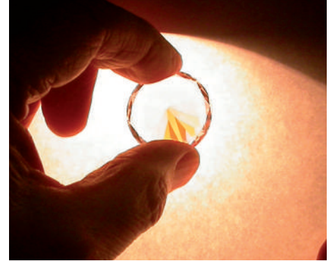
A large CZ showing the orange pavilion flash effect which is achieved by holding the table of the stone against a sheet of white paper placed close to a light source. The light fails to come through the stone completely, as it would with stones of lesser RI value. e.g. zircon or YAG. As the stone is tipped slightly, the whole of it becomes illuminated after a dispersive orange flash is seen. This is characteristic both for standard brilliant cut CZ and princess cut CZ. Photo by Gwyn Green.
