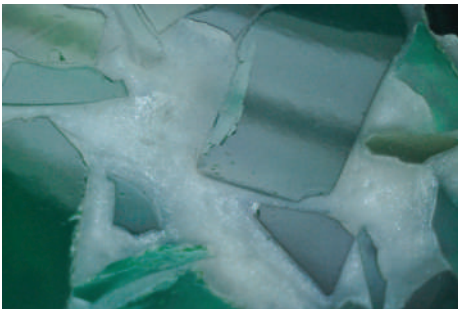
2: The green and white veined areas displayed distinct differences in lustre. Note the duller lustre of the polymer filled areas. Magnified 25x.
