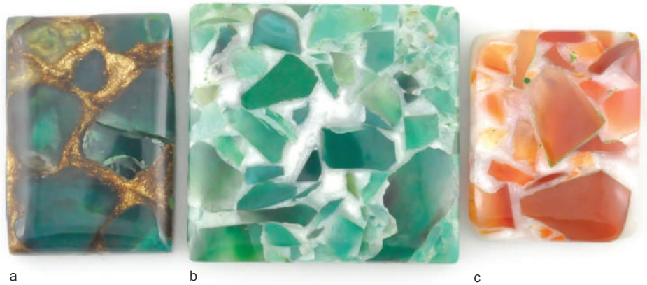
1: These three composite specimens, (a) dark green, (b) light green and (c) orange with golden and silvery white matrix, were made up of chalcedony pieces in a polymer matrix.
