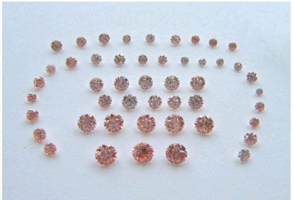
CVD-grown synthetic pink diamonds ranging from 0.01 ct – 0.27 ct). Photo by H. Kitawaki.
