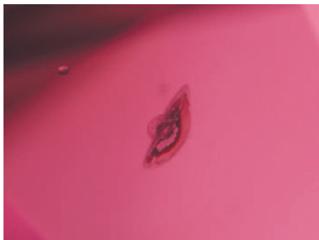
6: Rubies may be heated utilizing a wide range of temperature, time and other conditions. However not all inclusions will react to such heating at the same time/temperature, making the identification of certain kinds of heating (in particular those utilizing relatively lower temperatures) more difficult. Shown in this image are two mineral inclusions, one showing clear evidence of thermal alteration, whereas another in close proximity does not show any evidence of being altered.
