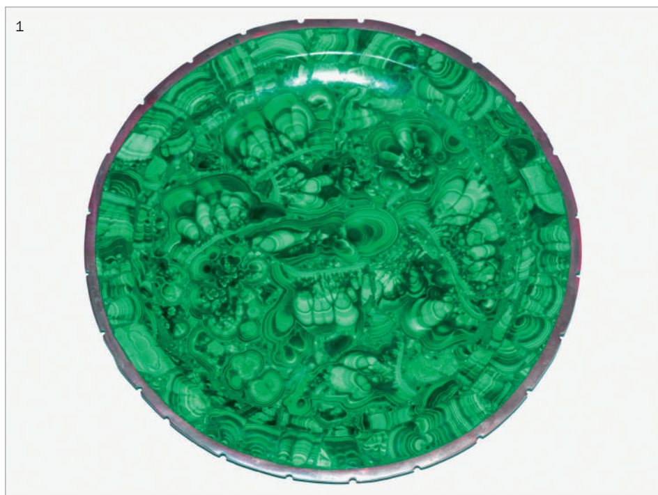
This plate weighing approximately 958 g proved to be made up of small fragments of malachite bonded or cemented together.
