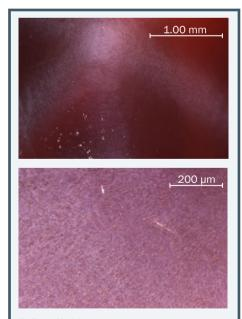
9: The off-white star on the upper curved surface of the ruby cabochon is caused by a network of oriented needles or fibres. Reflected light.
