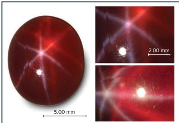
1: The star ruby submitted for examination shows two stars: an offwhite six-rayed star on the upper surface of the cabochon, and under slightly oblique fibre-optic illumination, an orange red star. In particular orientations, one or two of the off-white arms of the ruby are displaced by lamellar boundaries, particularly in two of the arms. Size of the stone is  $10.3 \times 8.7$  mm.
