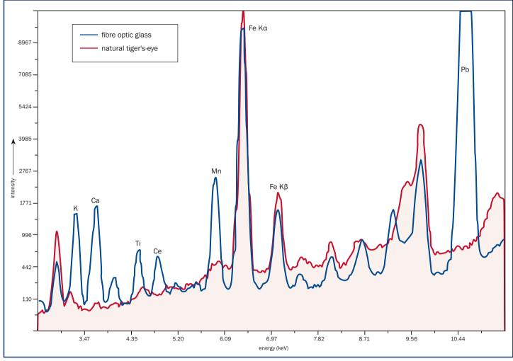
3: EDXRF spectra, comparing fibre optic glass with natural tiger's-eye.
