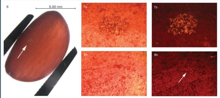
6: Irregular colour distribution at the surface of the ruby cabochon. The unpolished part of the cabochon contains several spots of foreign material (indicated by arrow). Immersion.
