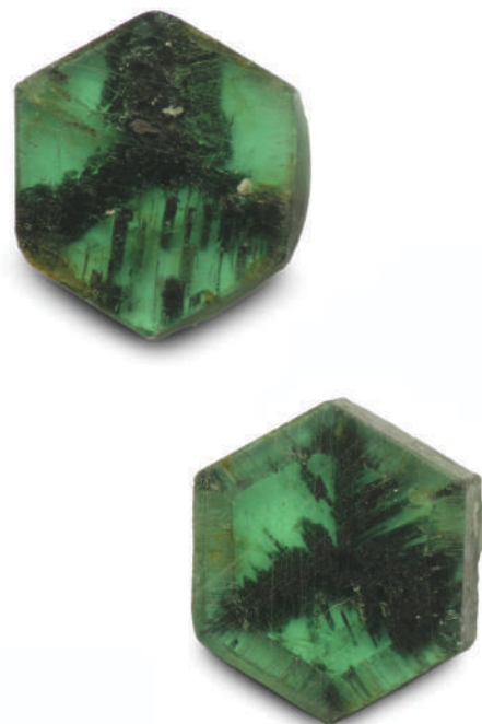
Above: Slices of trapiche tourmaline from Zambia cut perpendicular to the c-axis. View parallel to the c-axis, size of the samples about 13 × 12 mm. Photos by T. Hainschwang.
