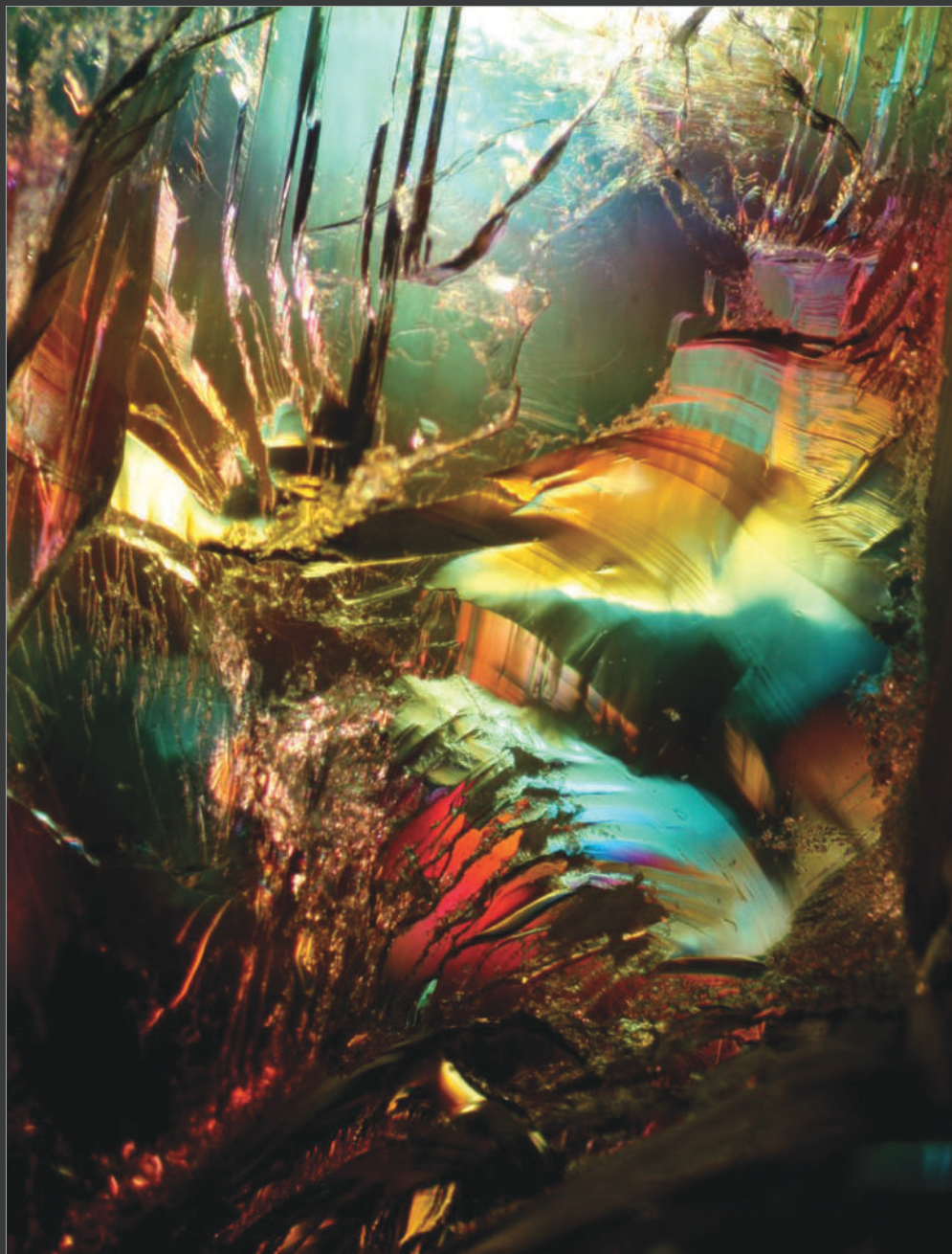
A zultanite (diaspore) crystal weighing 221.81 ct. In one area of the crystal I found a fracture surface that was beautifully enhanced by a thin film inclusion displaying vivid interference colours (right).
