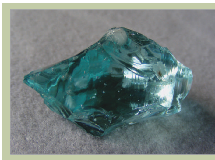
1: Blue glass of approximately 36 x 26 x 20 mm, with round gas bubbles visible with the naked eye. The two largest devitrification inclusions are at the top and towards the right-hand side.
