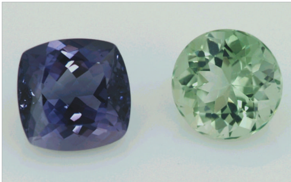
16: ‘Blueberry quartz’ (left) is produced by gamma irradiation and heat treatment of prasiolite (right). Photo: R. Schultz-Güttler, Sao Paulo.
