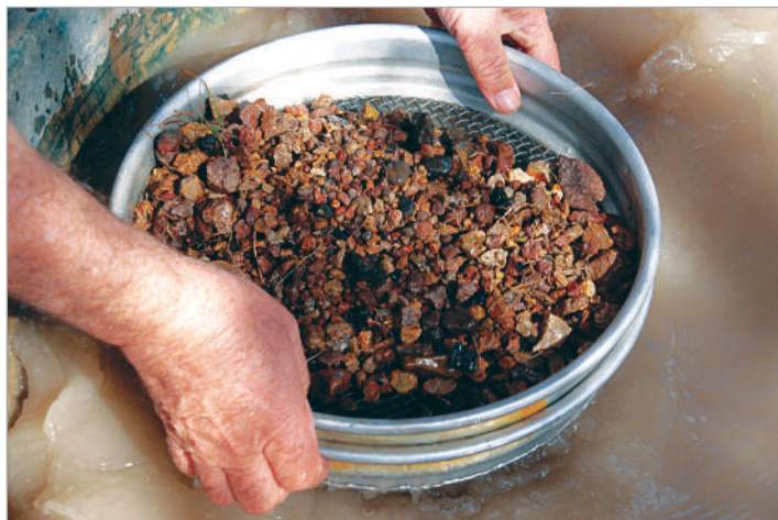
Washing and sieving sapphire-containing gravel at the Reddestone Creek fossicking area.
