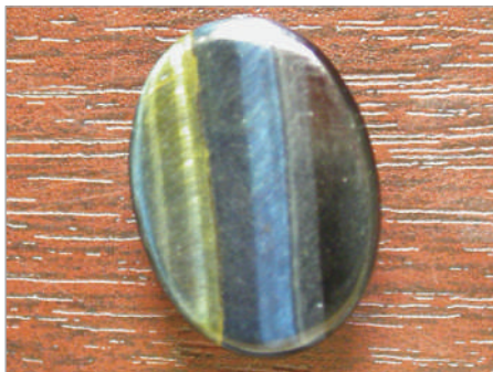
2: Base of tiger's-eye cabochon used for thin section. This shows bright bands and streaks. Length 17 x 12 mm.
