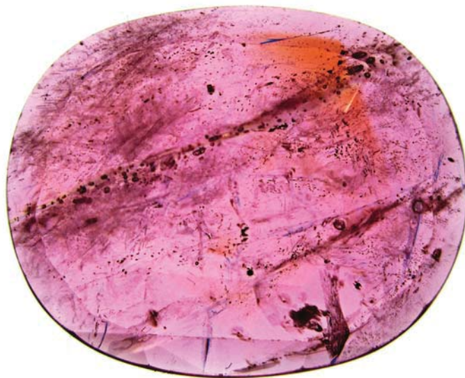
Purple colour flashes and bubbles in a lead-glass-filled ruby. Copyright Gem-A, photo by Jack Ogden.
