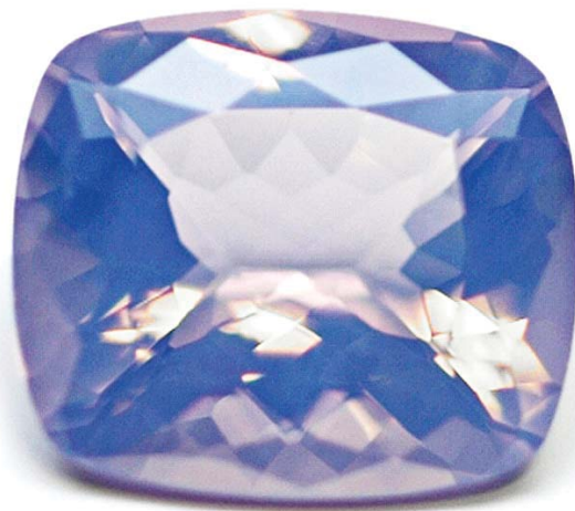
Faceted 'neon quartz', i.e. bleached amethyst. The milky appearance is produced by microscopic fluid inclusions, formed by heat treatment. Photo by German Gemmological Association.
