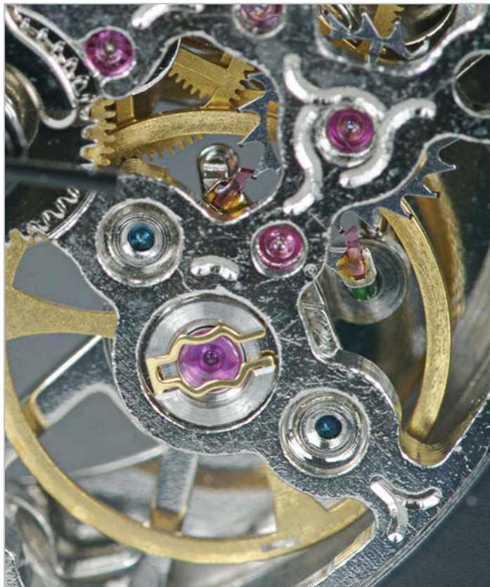
Jewel bearings used for a balance wheel in a modern mechanical watch movement. Photo by Hustvedt used under Creative Commons License, see http://creativecommons.org/licenses/by-sa/3.0/deed.en
