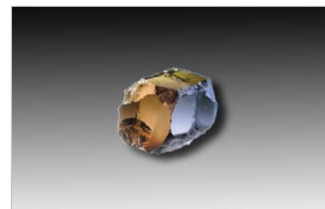
For one group of the natural-colour tanzanite, a strong trichroism with pleochroic colours of blue, purple and a mustard-yellow can help to identify unheated tanzanite, as seen in this oriented polished cube.
