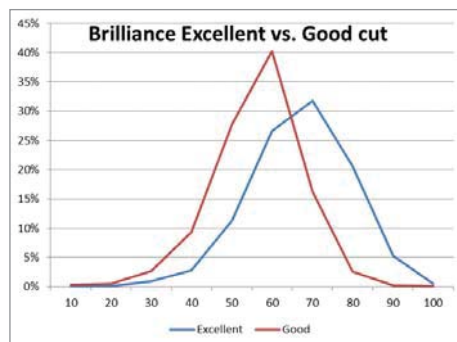
6. Brilliance as function of cut. Note that for a Brilliance level of higher than 70, there are 58% of the population with Excellent cut grade while in Good cut grade there are only 19% of the population.
