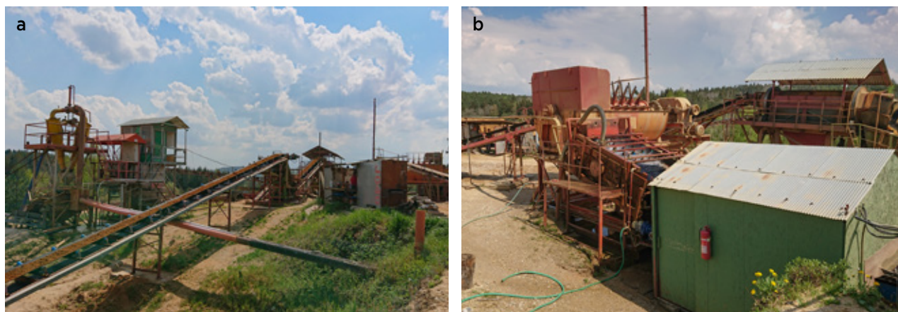
Figure 5: (a) The mined sediments are processed in this washing and sorting plant. (b) After screening out smaller size fractions, the moldavites are hand-picked in the green building. Photos by T. Stephan.
