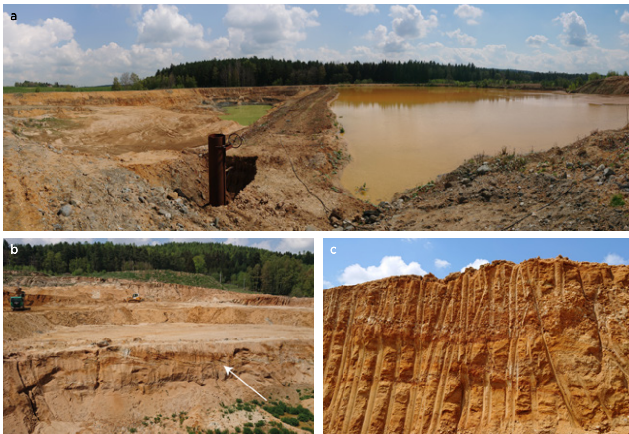
Figure 4: (a) The sand-and-gravel quarry near Chlum is expansive. The sediments lie on top of gneissic bedrock (exposed as the dark area on the far side of the smaller pit to the left). (b) Mining involves the use of excavators and trucks. A claystone horizon (indicated by the arrow) forms a darker brown layer in the pit wall in the foreground. (c) Moldavite is found in subhorizontal gravel layers. (The vertical lines are from the excavator used to mine the sediments.) Photos by T. Stephan.
