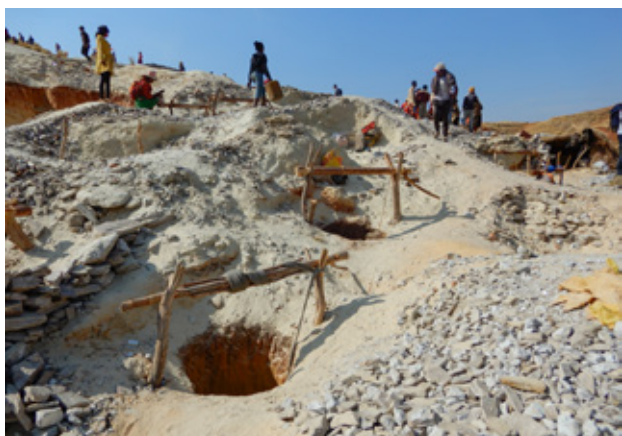
Figure 16: A closer view of the workings illustrates the simple techniques used by the miners, including primitive windlass systems. Photos by M. Novák.
