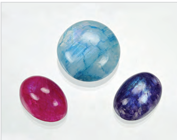
Figure 41: Sold as dyed rainbow moonstone, these cabochons proved to be labradorite that has been treated with organic dyes. The diameter of the light blue cabochon is 16 mm. Photo by S. Koch, DSEF.
