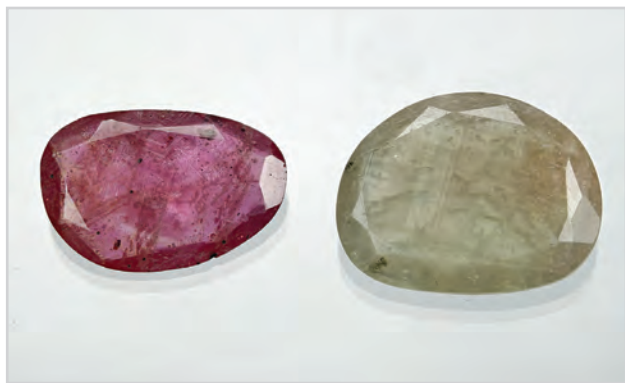
Figure 37: These faceted tablets of red and pale green corundum (6.03 and 10.41 ct, respectively) have been treated by coloured lead-glass fillings. Photo by S. Koch, DSEF.
