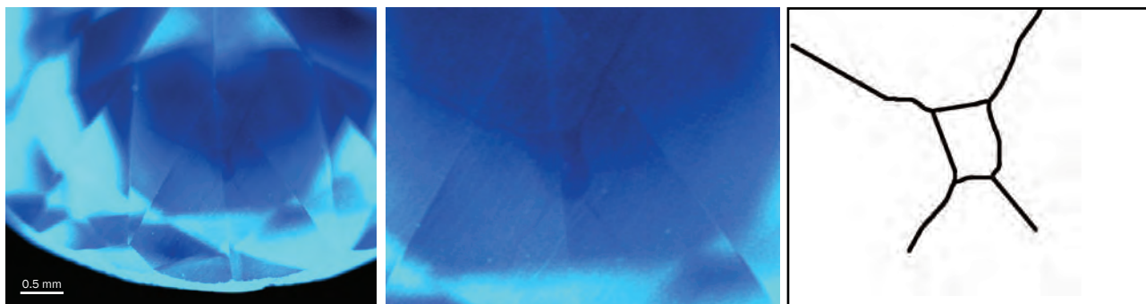
Figure 27: The DiamondView images of the 1.01 ct diamond show a luminescence pattern reminiscent of near-colourless HPHT synthetics, with a square core and four branches radiating from the corners. Photomicrographs and drawing by A. Delaunay.
