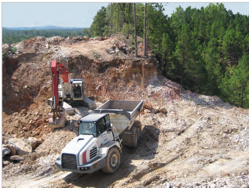
Figure 7: The McEarl mine is currently worked as an open pit with a trackhoe and dump truck. Photo by J. Zigras.
