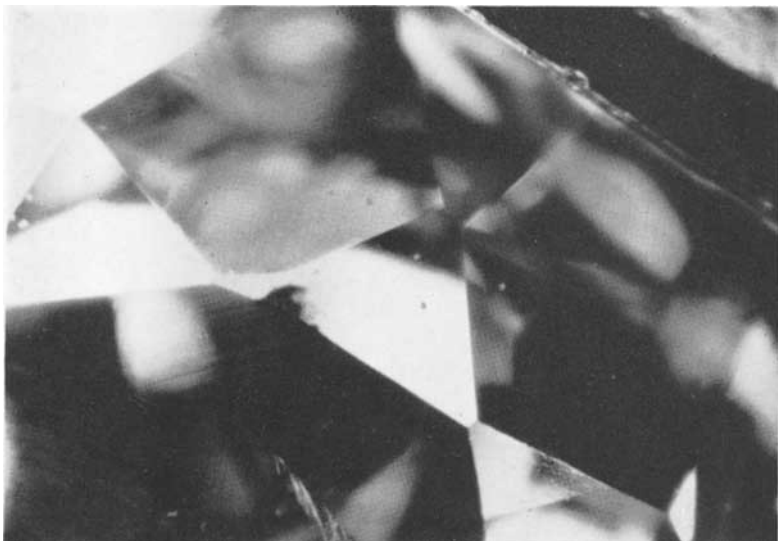
FIG. 5. Dark spots due to irradiation, at the angle of table and star facet, on diamond number 21. The depth of penetration is 0.03 mm and was better visible in reality. Magn. \times 25 .
