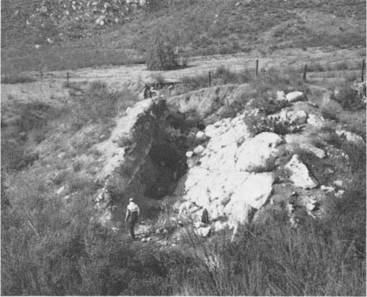
FIG. 5. Pegmatite dike at the Mack mine, Rincon district, San Diego County, California. The white area in the centre is the dike which is dipping 43 degrees southwest. This mine is noted for prisms of light-green beryl.
