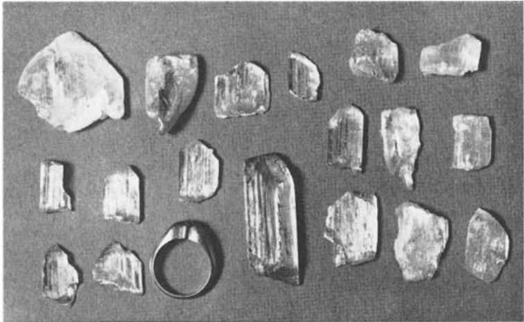
FIG. 9. Small crystal fragments of spodumene from San Diego County, California. The specimen in the upper left exhibits the typical etched termination on a crystal fragment. Notice the striations.
