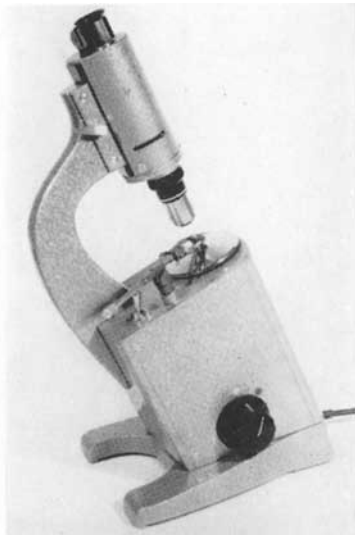
FIG. 3. Latest Gubelin model, with incorporated Zeiss spectroscope, to be used in transmitted or in reflected light. The additional lamp used in the second procedure is not illustrated.
