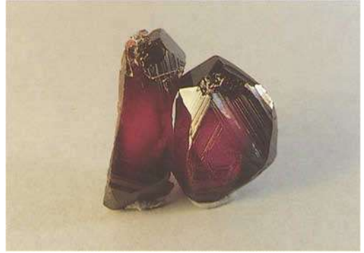
Fig. 12. Two synthetic ruby crystals with platinum wire protruding.
