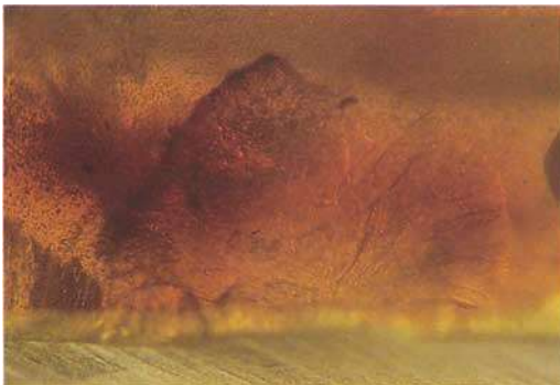
Fig. 15. A flaw in the amber of Figs 13 and 14 which resembles the stress figures seen in much clarified amber.
