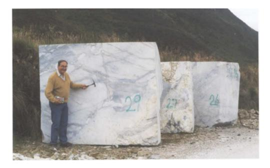
Figure 5: Ledmore marble quarry. Slabs of grey architectural marble showing typical deformation textures. Photo by Douglas Nichol.
