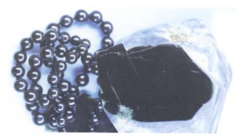
Figure 4: Rough inky omphacite jade and polished beads of the same material.
