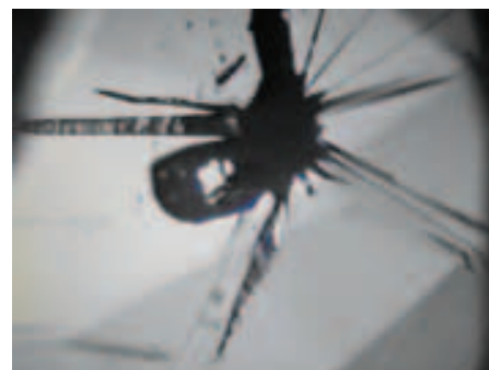
Figure 5: Inclusion typical of spinel from this locality in which a probable cavity is at the centre of a radial array of empty channels. The width of the field of view is 3 mm.
