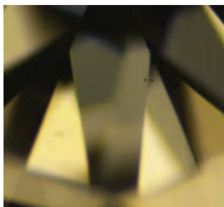
Figure 2: Dark inclusion in a 0.56 ct CVD synthetic diamond, Magnified 50 ×. Photomicrograph by Zhonghua Song and Licong Li.
