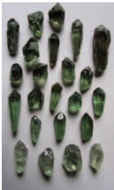
Figure 24: Gamma-irradiated green quartz from Rio Grande do Sul, Brazil. Although the irradiation dose is the same, the difference in colour of the crystals from pale green in the lower left to dark green in the upper right is clearly visible. Size of specimens from 1.5 to 4.6 cm. Photo by Rainer Schultz-Güttler.
