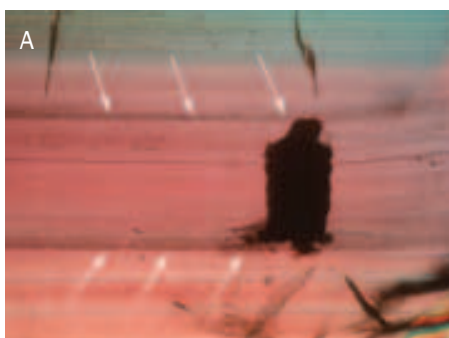
Figure 31: Growth boundaries showing somewhat irregular, 'cobbled' surfaces which are caused by some dissolution at the beginning of each growth cycle; occasionally, numerous small particles (indicated by arrows) are trapped close to some of these irregular surfaces. (A) seed confined to the outer layers by two irregular surfaces, (B) numerous irregular surfaces at successive growth boundaries, (C) numerous irregular surfaces at successive growth boundaries, one of them with a high concentration of trapped particles.
