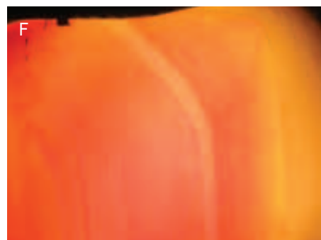
Figure 30: Characteristic interference patterns displayed by the layered growth structures of a faceted synthetic alexandrite.
