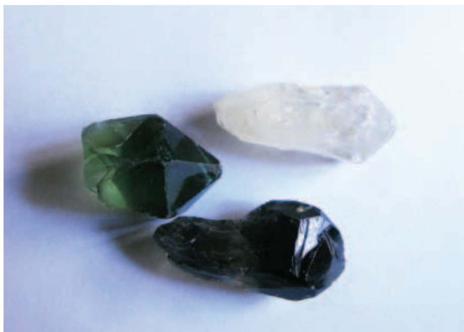
Figure 27: Untreated and gamma-irradiated wet quartz crystals. The same dose of irradiation produces different intensities of colour. Size of specimens between 2 and 4 cm. Photo by Rainer Schultz-Güttler.
