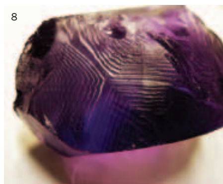
Figure 6: Two amethyst cross sections indicating different colour intensity in different growth sectors. Sectors of the positive rhombohedron r possess more intense violet colours compared to sectors of the negative rhombohedron z . Size of specimens 2.5 and 2 cm. Photo by German Gemmological Association.
