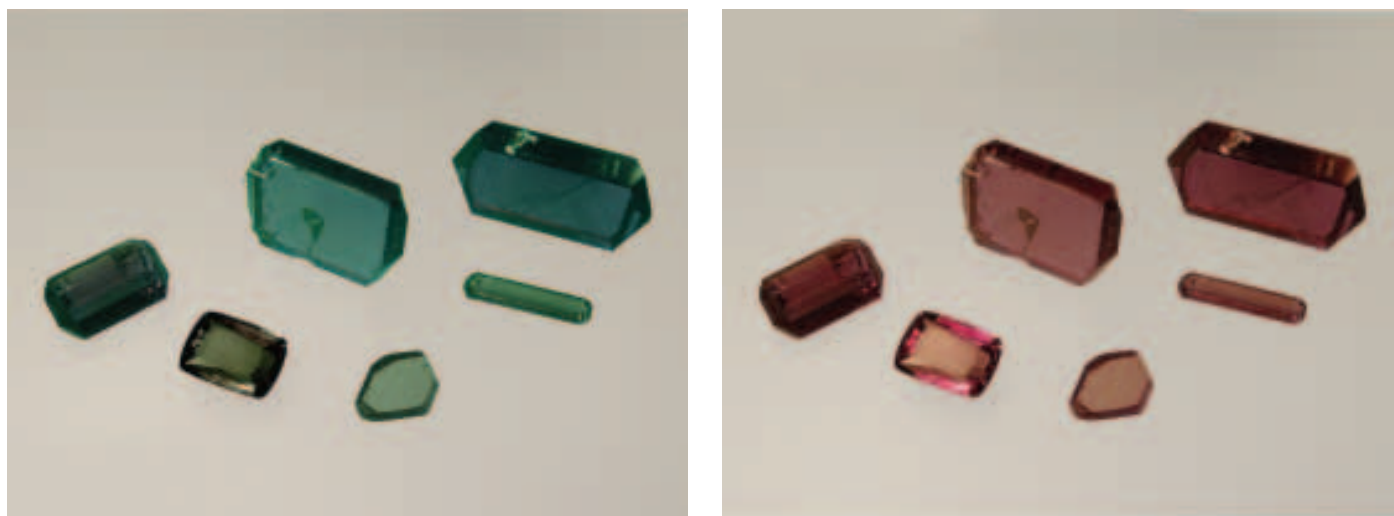
Figure 5: Different types of rough and faceted synthetic alexandrites grown by Creative Crystals Inc. in daylight (left) and incandescent light; the crystals were grown on seeds parallel to the b pinacoid (1,2), parallel to the r prism (3,6) or parallel to the l dipyrmaid (4); the faceted alexandrite of 13.49 ct measuring 16.6 × 11.8 mm (5) was grown on a seed parallel to the r prism. Photo by K. Schmetzer.
