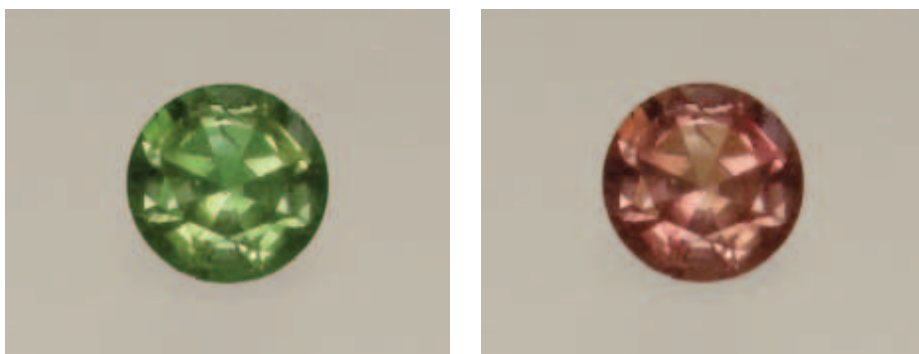
Figure 1: One of the first synthetic alexandrites grown by Creative Crystals Inc. in the early 1970s in daylight (left) and incandescent light (right); diameter of the sample 5.5 mm. Photo by K. Schmetzer.
