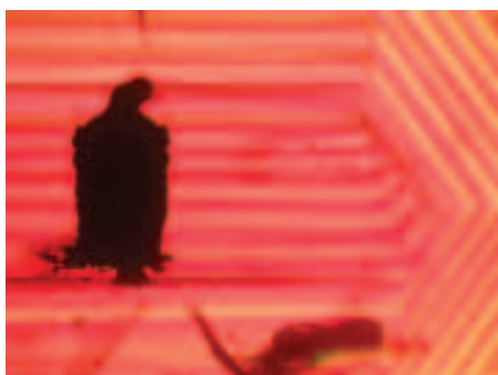
Figure 29: Growth zoning, associated with colour zoning in a synthetic alexandrite crystal grown with r seed orientation, growth zone [310], faces r and l ; from the centre to the rim, each growth layer starts with an intensely coloured area which gradually fades to a paler zone and then to a near-colourless part.
