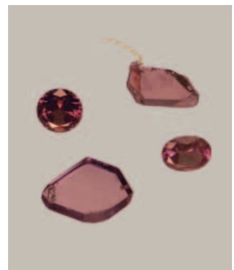
Figure 25: Rough and faceted synthetic alexandrites grown with seeds which were cut parallel to the l (133) prism in daylight (above) and incandescent light (below); the crystals (see Table I) weigh 5.15 ct (lower left) and 3.08 ct (upper right); the faceted stones weigh 2.43 ct (upper left, diameter 8.4 mm) and 1.91 ct. Photos by K. Schmetzer.
