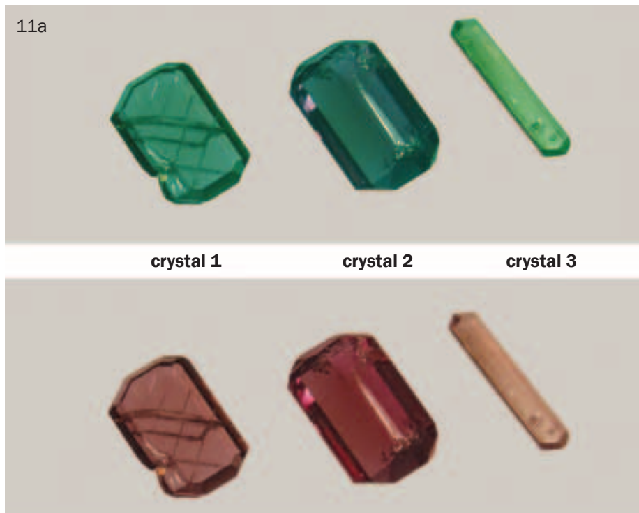
Figure 11: Morphology of three crystals grown by Creative Crystals Inc. with r (130) seed orientation (crystals 1 to 3 of Table I). (a) samples in daylight (above) and incandescent light, size of the right columnar crystal 22.8 x 5.2 mm (samples to scale); (b) crystal drawings in parallel projections in views along the c -axis (left column) and photomicrographs of the samples in identical orientations in immersion (right column, samples not to scale). In the sequence of crystal 1 to crystal 3, the way in which the face parallel to the r seed grows and becomes gradually smaller with a , b and m faces becoming larger is visible. In crystal 3 the r faces parallel to the seed are comparable in size to the r faces which are not parallel to the seed. Photos and crystal drawings by K. Schmetzer.
