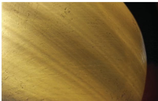
Figure 5: Viewed with transmitted fibre-optic illumination, this close-up of specimen D (22.5 g) reveals the layered structure of the Tridacna shell from which it was cut. Photo by M. S. Krzemnicki, © SSEF; image width 11 mm.
