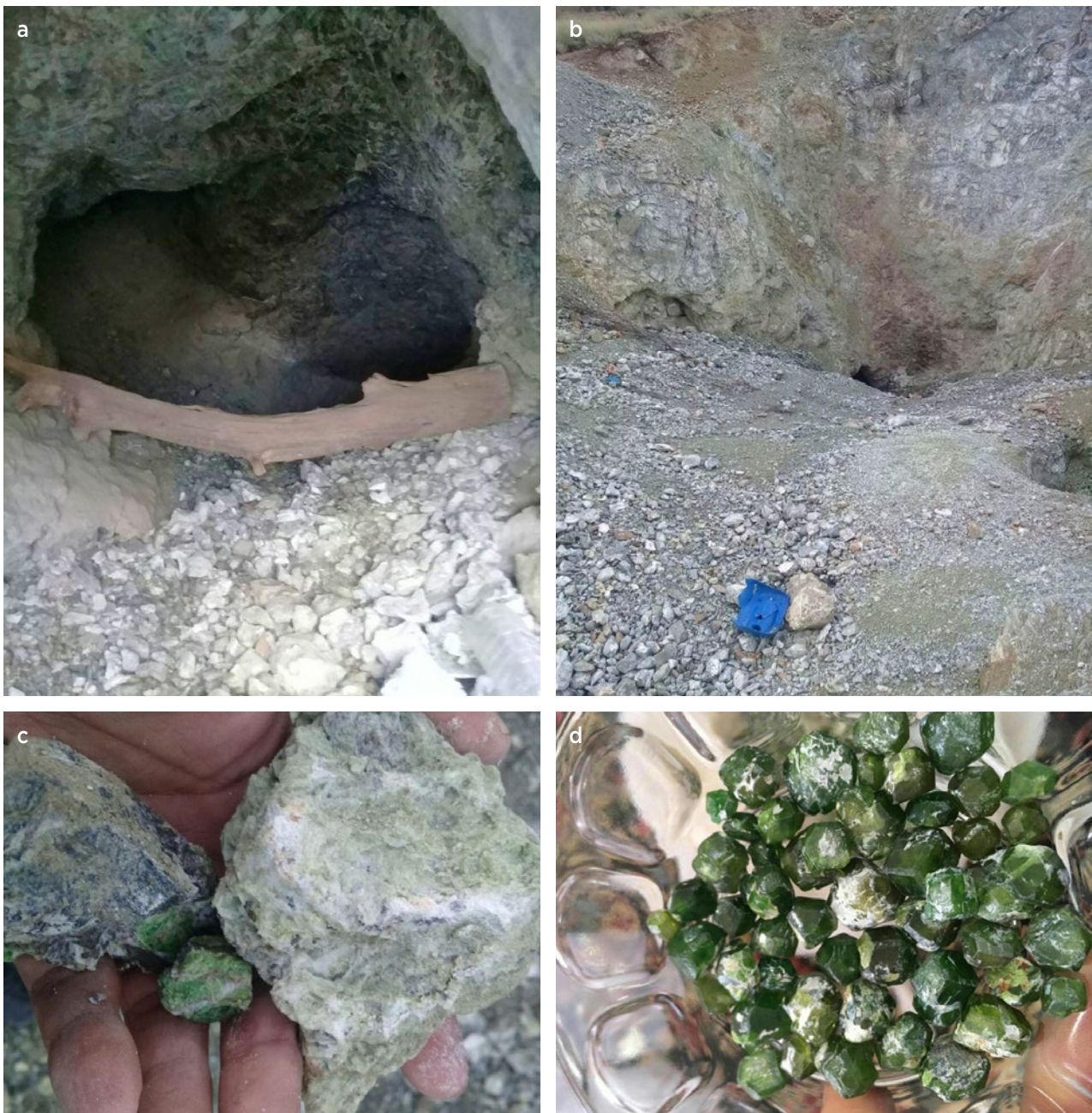
Figure 3: (a, b) Demantoid mining near Bagh Borj has been done in tunnels and open cuts excavated by local residents. The underground workings can reach more than 50 m. (c) Demantoid is hosted by weathered serpentinite and is easily separated from it. (d) These demantoid crystals average 1 g each. Photos by V. Ahadnejad.
