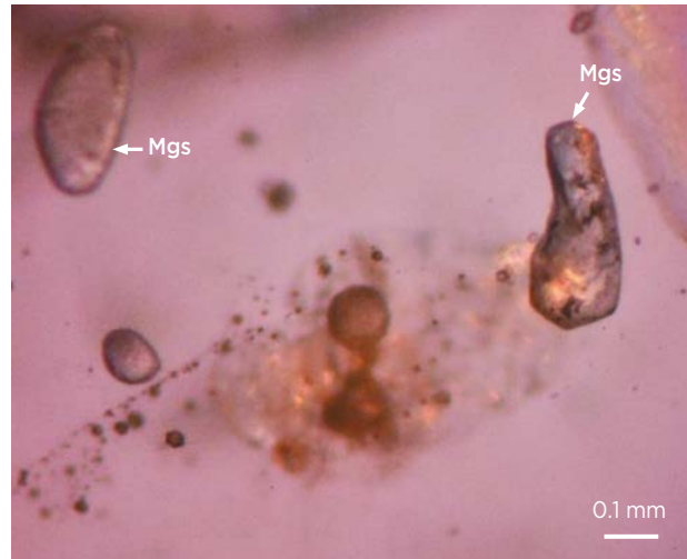
Figure 6: An example of carbonate inclusions observed in the Mogok spinel samples is shown here by magnesite (Mgs). Photomicrograph by M. M. Phyto.
