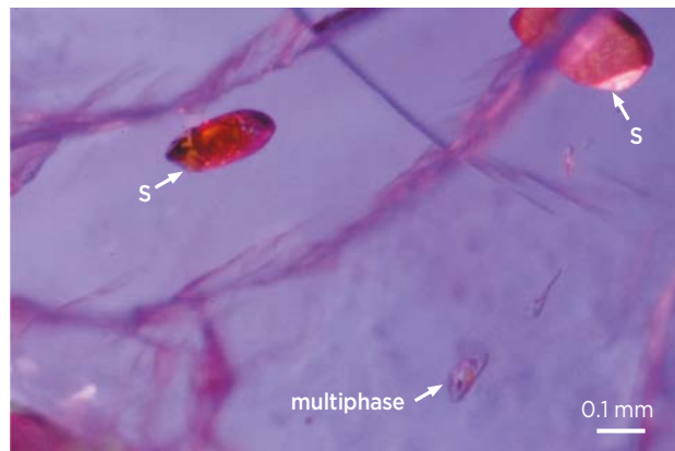
Figure 11: Solid inclusions of elemental sulphur (S) are seen here with multiphase fluid inclusions (probably containing liquid and sulphur) in a spinel from Mansin. Photomicrograph by M. M. Phyto.
