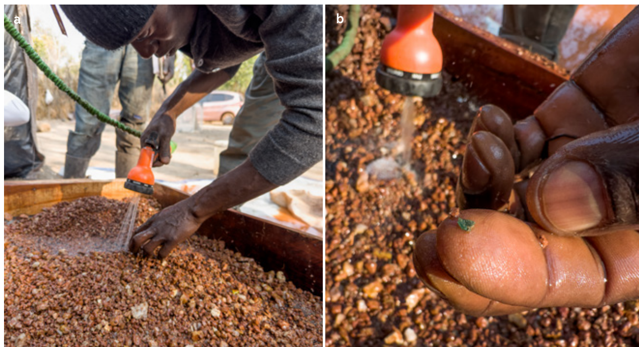
Figure 9: (a) The gravels are then washed on fine-meshed screens, and (b) the emeralds are removed by hand. This emerald (about 5 mm long) was acquired for the LFG reference collection after the authors witnessed its recovery by the miner. Photos by V. Pardieu.
