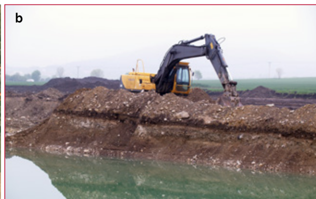
Figure 5: (a) An aerial view (from www.mapy.cz ) of the Podsedice mining area in the Central Bohemian Highlands shows the locations of (1) the present mining area and (2) the treatment plant. (b) At Podsedice, overburden is removed and garnet-bearing gravel is extracted from open pits using an excavator. Photo by Aleš Hladký.
