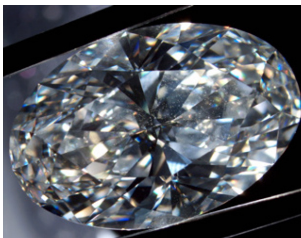
Figure 27: This 10.97 ct diamond with E colour and IF clarity would be expected to be type IIa, but revealed weak type IIaA nitrogen features in its infrared spectrum. Photo by A. Delaunay, © LFG.
