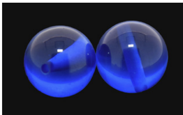
Figure 33: These two beads (18.1 ct each), imitating Co-blue spinel, were found to consist of coated synthetic sapphire. Photo by S. Li.
