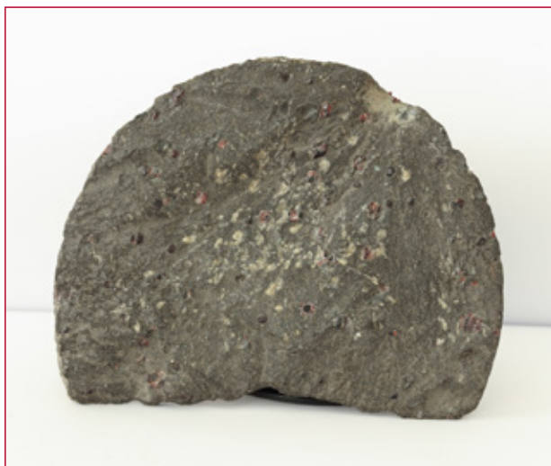
Figure 4: A drill core from Linhorka, Central Bohemian Highlands, Czech Republic, shows the presence of Bohemian garnets in serpentinised garnet peridotite. The sample measures 12 cm across and is from research drill hole T7, obtained from a depth exceeding 209 m. Photo by Aleš Hladký.
