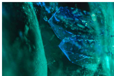
This photo shows two quartz crystal inclusions that have broken the exterior surface of a Colombian emerald. A filler that fluoresces blue under long-wave UV (LWUV) light was used to enhance the clarity of the stone and flowed in around the quartz structure. The result is a photo that vividly displays the contours of the quartz inclusions in a blue fluorescence when LWUV light is shone onto the emerald. Photo by Jacob Martin, field of view 1.99 mm.
