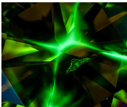
Telltale fluorescence sectoring accompanied by a magnetic metallic flux inclusion in an high-pressure, high-temperature lab-grown diamond. The specimen was photographed in 365 nm UV illumination. Photo by Randy Lightfoot, field of view is approximately 5.00 mm.
