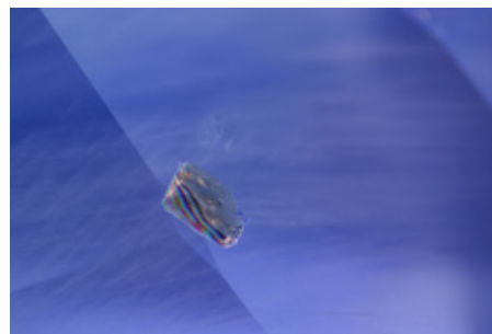
A biotite crystal in an untreated Sri Lankan blue sapphire. The image on the left was captured under native lighting conditions, while the right-hand image was recorded with polarisers applied, revealing vivid interference colours. Both photos were captured with a Leica S9D and Canon EOS RP under darkfield and fibre-optic illumination. Focus stacked; field of view: 3.5 mm.
