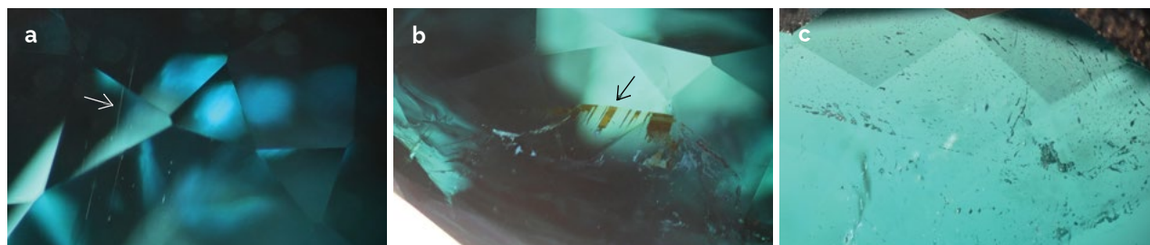
Figure 6: Additional internal features observed in faceted Ethiopian Cu-bearing tourmalines include (a) fine hollow needle-like structures oriented parallel to the c -axis, (b) planar channels partially filled with an Fe-rich substance and (c) a network of irregular fluid inclusions, locally developed as ‘trichites’. Image a shows ETH_3, for which the treatment status is unknown; images b and c depict ETH_13, reported as heat treated. Photomicrographs by SSEF; magnified 50 \times .
